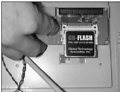
Mount the GB-Flash module inside the system case
